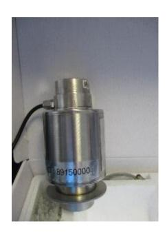
To make sure that all the cells are correctly configured, go to the step Calibration >> Scale selection >> Serial number configuration >> Digital cell configuration. A message with wrong or correct cell configuration will be shown.
